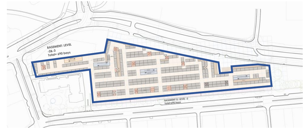
Basement Parking Level -2 & -3 Approximately 690 parking bays per level
