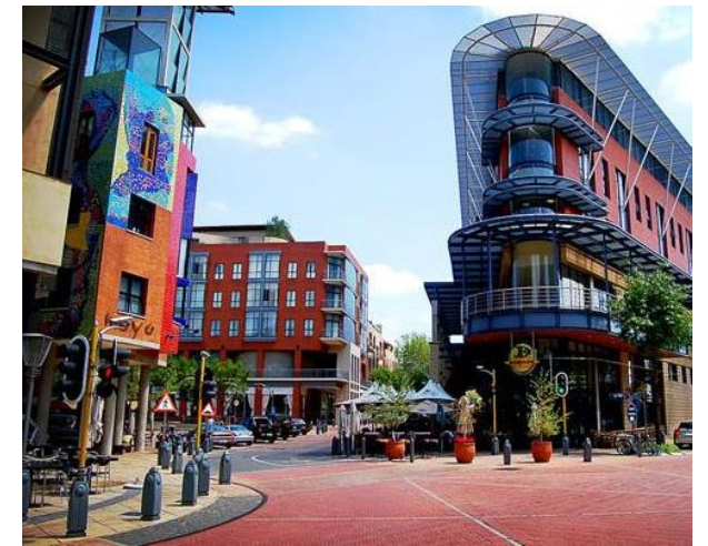
Raised and Paved Intersections as well as wide sidewalks to accommodate restaurant/retail spill out at Melrose Arch, Johannesburg.
