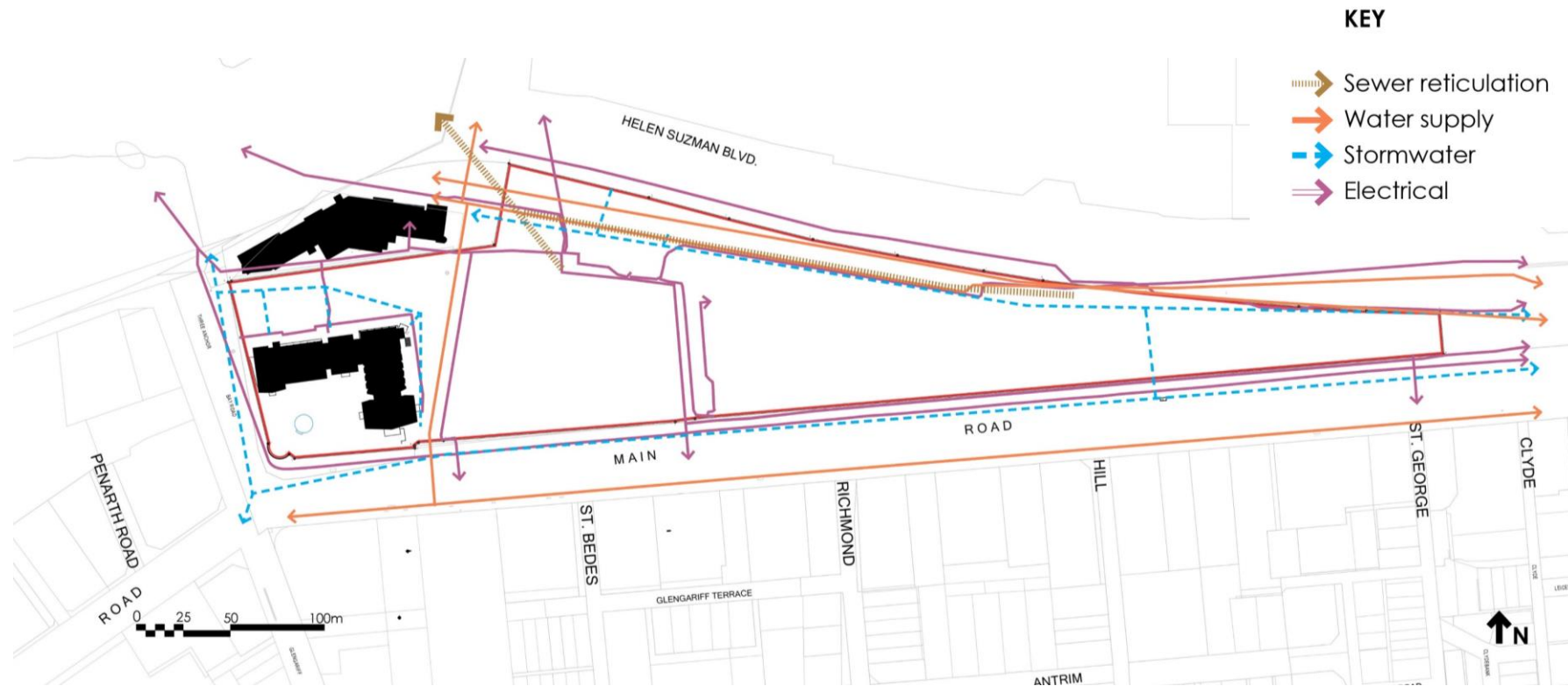
Existing civil services on the site.
