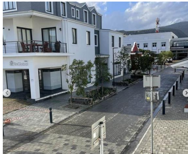
Bollards and change in paving texture in Hermanus by Gapp Architects
